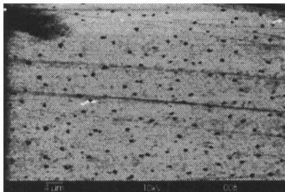
FIGURE 1 Scanning electron micrograph showing a representative top-view of a PDLC film
